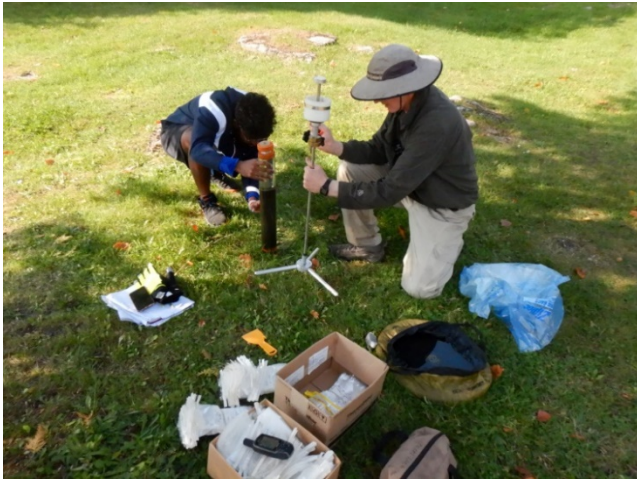
Preparing the equipment for the tedious job of extracting the core sample one quarter of a centimetre at a time
